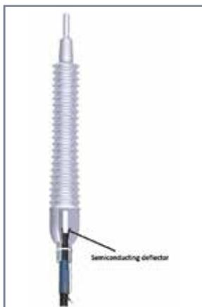
Fig. 1: Schematic of flexible dry-type outdoor termination.
